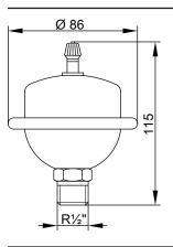
If the pipework to which the Vitodens is connected also supplies draw-off points at which water hammers may occur (e.g. pressure washers, washing machines or dishwashers): Install shock arrestors near the source of the water hammer (recommended). Flexofit S made by Flamco-Flexcon
